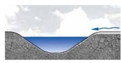
Vegetated Swale: These are used to remove soil particles and move stormwater through buffer strips and bioretention systems. Swales utilize land flow and mild
