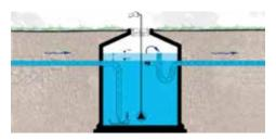
Cistern: These function mainly as rainwater storage and secondly for stormwater detention. The basic storage volume depends on the demand of rainwater use for
